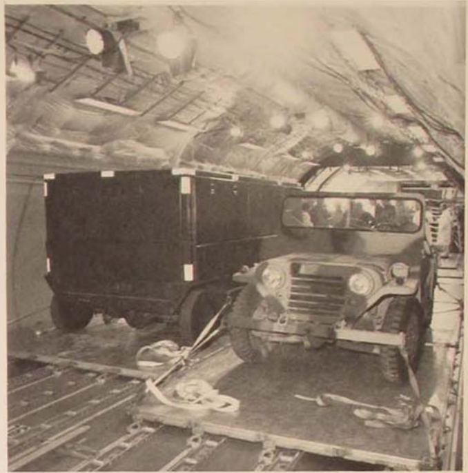
The KC-10A military tanker/cargo aircraft has essentially the same main deck in-plane cargo system as the DC-10 civil convertible, including side guide rails and end locks. It can also handle a civil air-cargo pallet.
