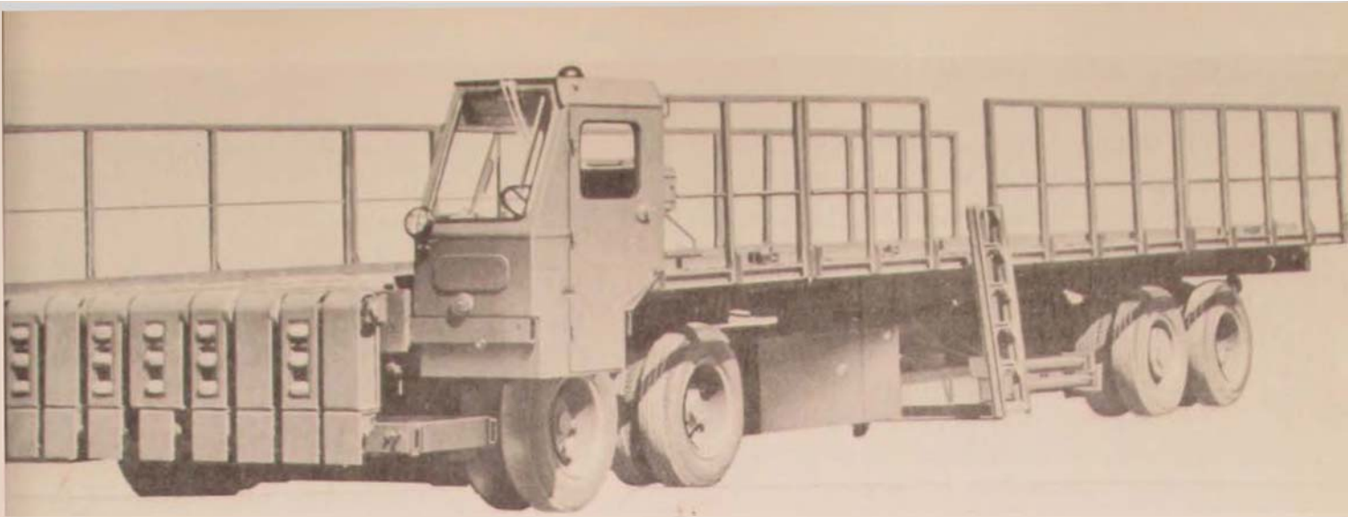
The 40K-Transporter Loader can elevate a maximum load of 40,000 pounds to a height of 13 feet.
