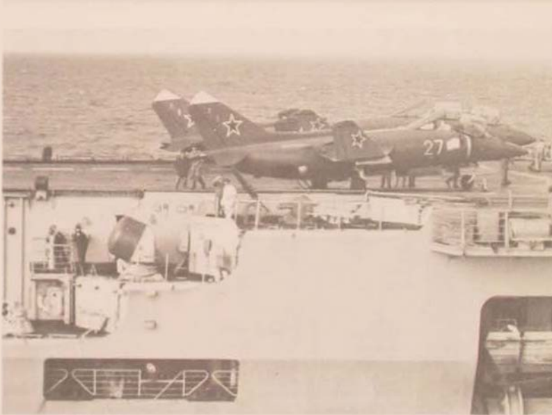
The Il-38 May (top), an antisubmarine maritime patrol aircraft, became more evident during the midseventies. . . . The variable-geometry, twin-jet bomber, the Backfire (middle), is replacing the Badger in the Soviet naval aviation inventory. . . . The Yak-36 Forger (bottom), a VTOL aircraft, is part of the weaponry of the Minsk-class aircraft carriers. About 18 Forgers are on each carrier, well armed with rockets, machine guns, bombs, air-to-surface missiles.
